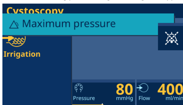
Excess pressure alarm
